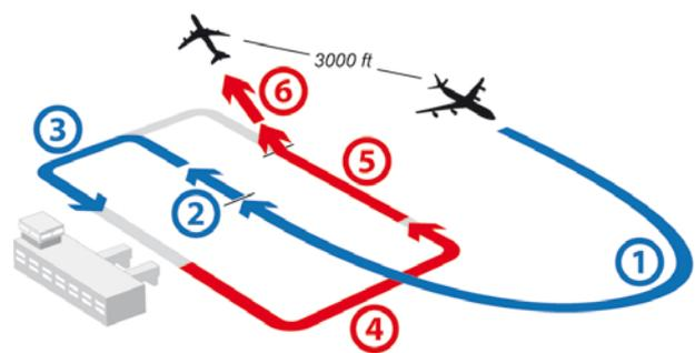
6 phases with climb out being split into (5) initial climb (lift off to main throttle back) and (6) final climb (throttle back to 3000 ft) and approach split into (1) approach to touch down and (2) touch down to end of rollout. (3) Taxi-in and (4) taxi-out stay the same.
