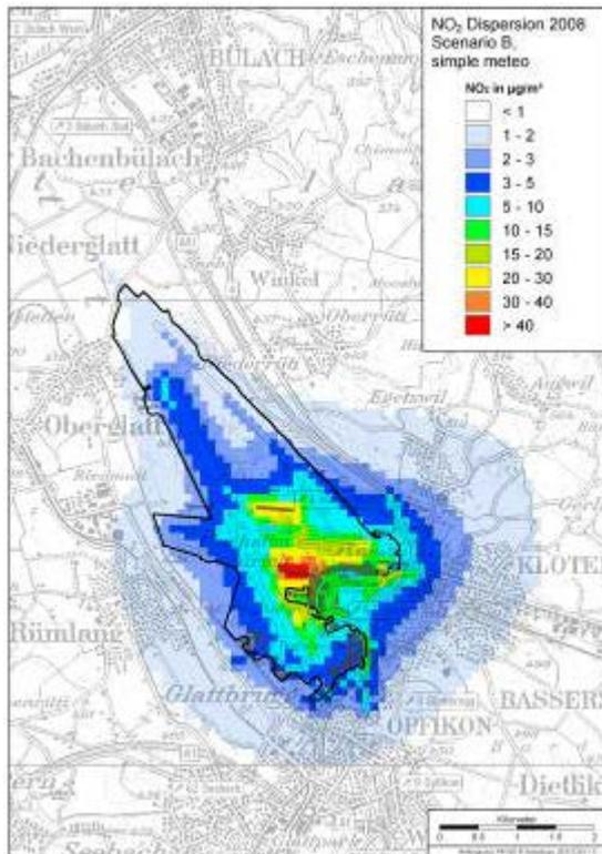
Figure 9 Scenario B concentration distribution using a modelled simple meteorology.
