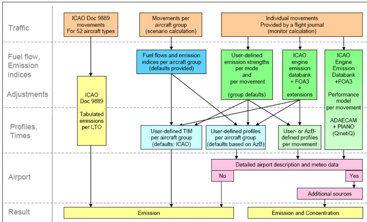
Figure 1 LASPORT aircraft calculation methods
