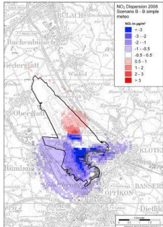
Figure 10 Difference between the simple modelled and actual meteorology for Scenario B.
